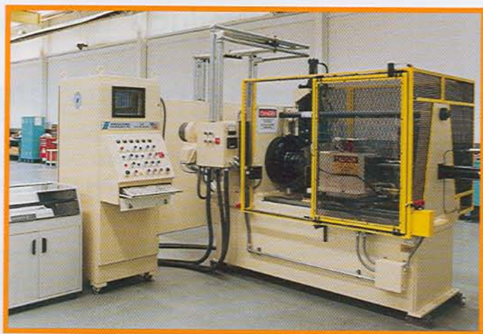
Fig. 8—A modern direct-drive friction welding machine, complete with computer controls, DC drive, and flash removal.
