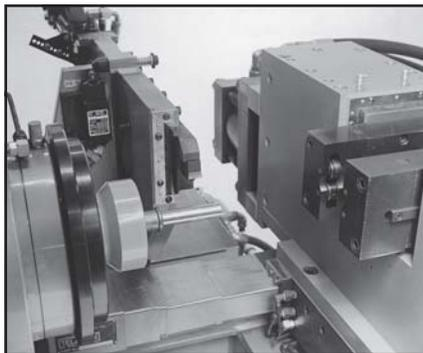
Above right: Model 150B Inertia Welder equipped with plunge-cut flash removal.
