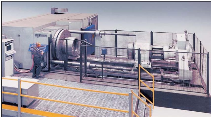
Model 400S Inertia Friction Welder
