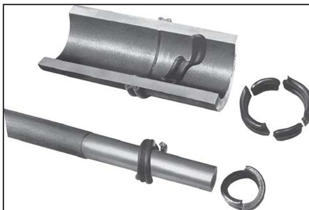
Right: Examples of I.D. and O.D. flash removed by shearing.
