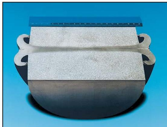
Transition joint for cryogenic application. Inconel to aluminum.
