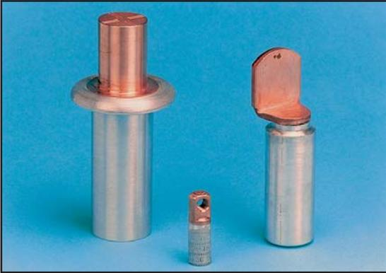
Metal combinations not normally considered "weldable," such as these copper to aluminum electrical connectors, can be joined in friction welding.
