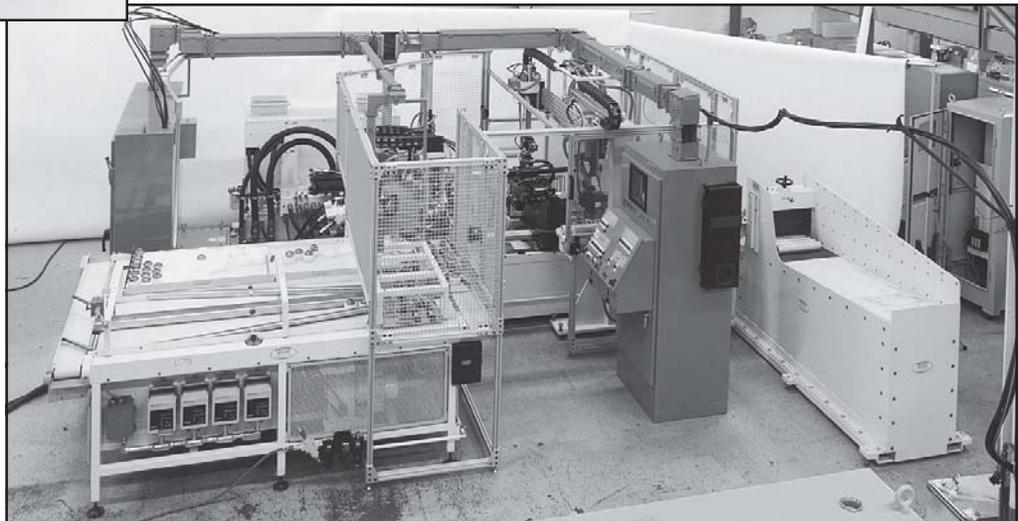
This twin welder has two independent spindles and fixtures to weld two solid ends to a hollow tube simultaneously. This welding cell includes automated spindle and fixture loading, flash shearing, flash removal conveyor, and part unloading conveyor. Welded assemblies are ready for fabrication and finishing. Production rates (dependent on tube diameter and wall thickness) are 250–300 welded assemblies per hour.
