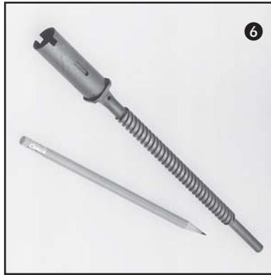
8 Stator vane adjustor lever-titanium.
