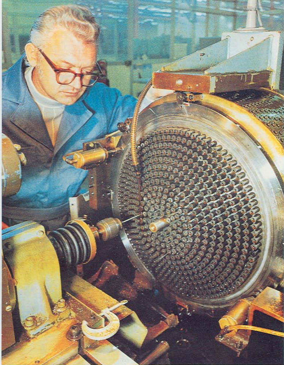
Injector stubs on main-injector base plate are drilled in preparation for welding of injector posts. Note tiered concentric-ring arrangement of the 600 stubs
