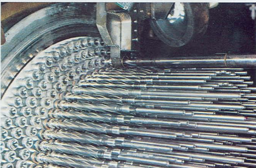
Drive bar on inertia welder (shown slightly retracted) is steadied by guide bushing. Serrations on post help grip drive bar. Guide rings on stubs will be removed
